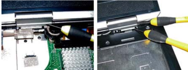
Fig. 20 Removing the hinge cover
